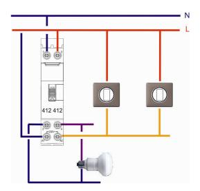
. 4 "NO" pulse operated latching relay
